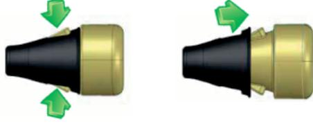
Cushion disassembly for cleaning and inspection of holders
